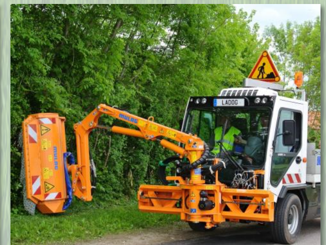
LADOG T-1550 with outrigger mowing head. The switchable pendulum front axle lock provides outstanding lateral ability and guarantees professional results.
