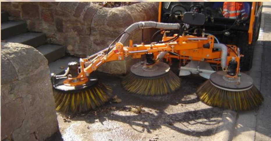
LADOG T-1150 with brush unit and a third brush for use on narrow walkways and in other particularly narrow areas
