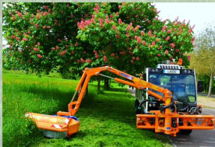
LADOG T-1550 with outrigger mowing head. The switchable pendulum front axle lock provides outstanding lateral ability and guarantees professional results.
