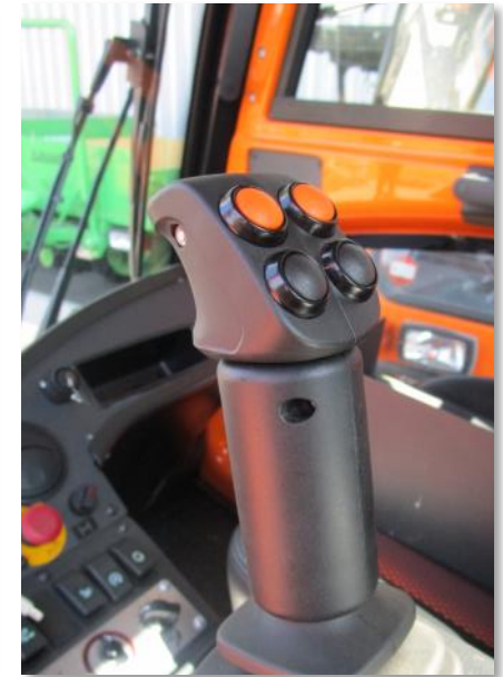
Various control options are available for operating the hydraulic functions
