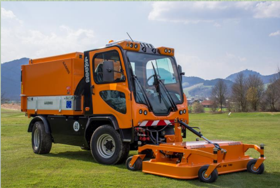
A classic tried and tested application. LADOG T-1400 with front rotary mower and collection container on the deck. Clippings are collected through the LADOG middle channel technique.
