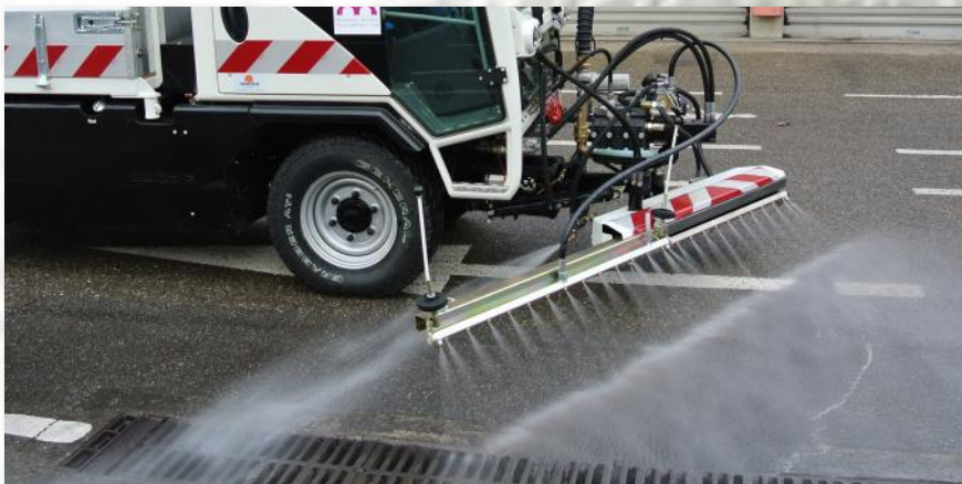
LADOG T-1250 with Jet-nozzle-system
