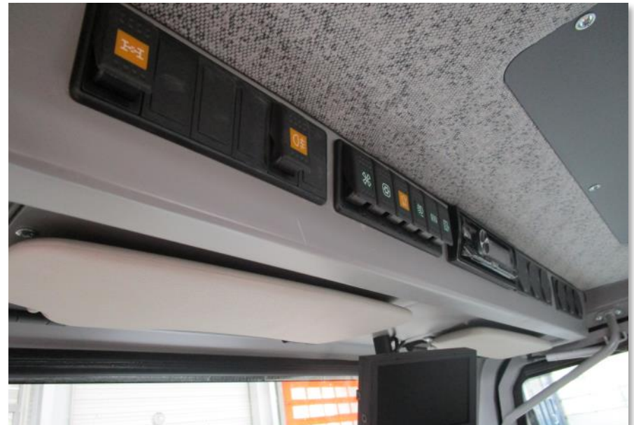
Various function switches, radio, odometer, etc. are clearly laid out and easily accessible in the overhead console
