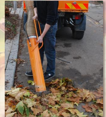
Flexible suction with the optional manual vacuum hose
